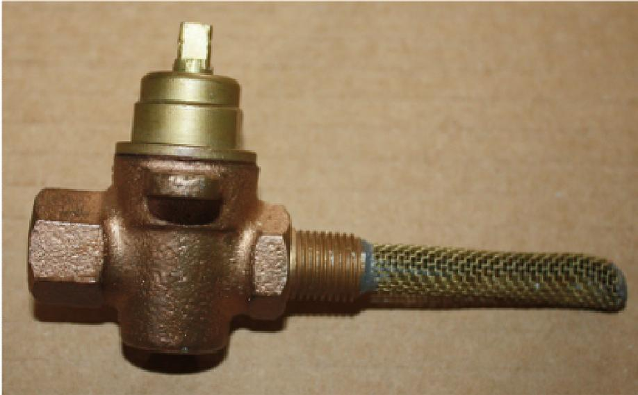
This is a photo of an earlier model of the fuel valve used in Champs. Aeronca introduced the use of this model valve in the early 40's. This valve has an inlet screen soldered onto the valve body. The valve body has 1/4" male straight pipe threads on the inlet and 9/16"-20 straight female threads on the outlet. The outlet is designed for a special tubing nut and feral. The valve body has "ears" on each side drilled for
