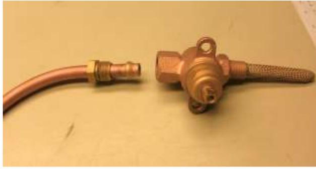
Bill Pancake took the three photos shown above. These photos are of a new valve and outlet nut and feral. The nut has non-standard 9/16 – 20 threads. According to Bill, at one time this nut and feral could be purchased at the local hardware store, but they are now difficult if not impossible to find.
