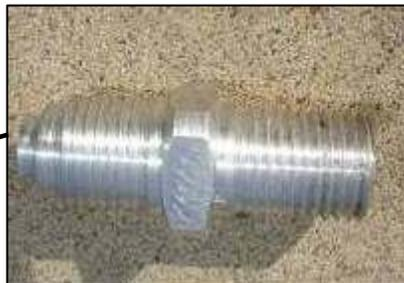
The photos above shows a transition fitting fabricated to convert to a flared copper fitting.
