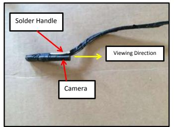
This is a photo of the camera with the cord bent back on itself and taped to the camera. You can also see a portion of the Solder used as a handle on the camera. The handle can be bent to position the camera below the exhaust valve after inserting the camera into the plug hole. It is important to minimize the overall diameter of the camera and handle as the assembly must be inserted into the spark plug hole.
