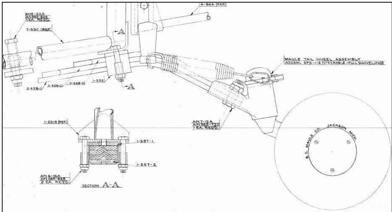
This figure shows a portion of drawing 4-620. It shows the mounting of the spring assembly to the airframe, provides reference part numbers to various components of the assembly, indicates the correct bolts and associated hardware for installing the tail wheel assembly and in section A-A provides details on how to clamp the spring assembly to the airframe.
