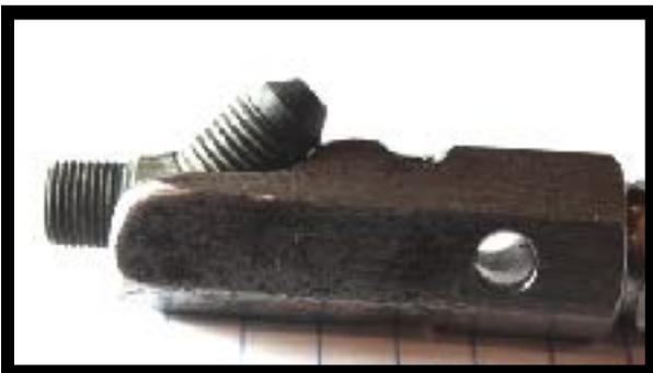
The next photo shows the 45degree fitting inserted into the slot in the end of the tool. When using the tool to insert the fitting into the engine crankcase, masking or electrical tape can be used to hold the fitting in position.
