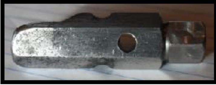
This photo is a side view of the tool. A 5/8" hex approximately 5/8" long is machined into the opposite end of the tool. Either a 5/8" socket or a 3/4" socket can be used to guide and drive the tool.
