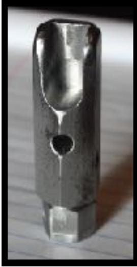
The tool also has two 1/4" diameter holes located approximately 1 1/4" and 1 11/16" from the slot end of the tool. These holes can be used to rotate the tool with a round rod handle.
