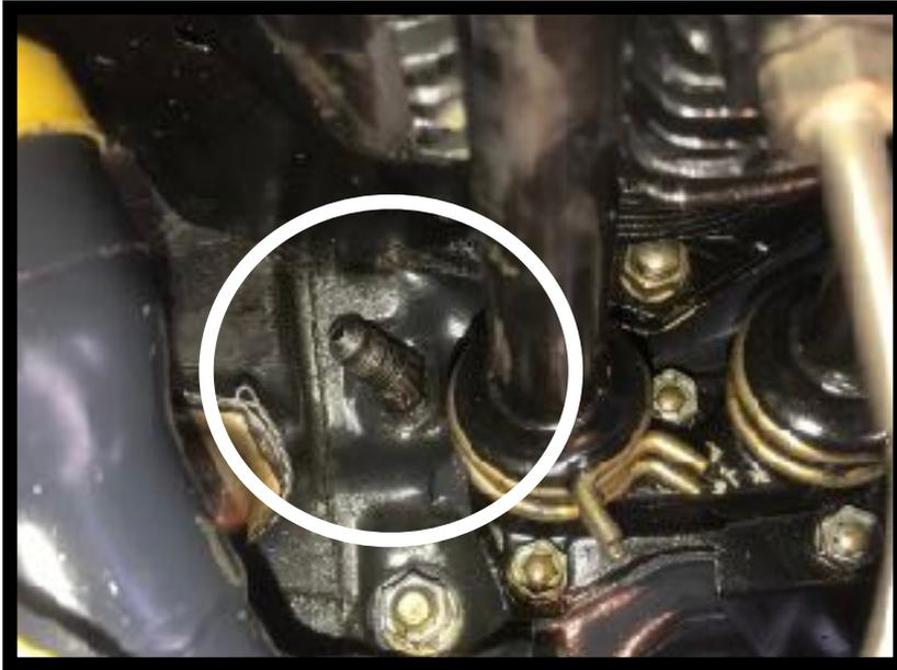
often has a brass orifice mounted in the fitting with an .040" restriction orifice hole. This line typically connects to the oil pressure gauge on the instrument panel. The photo on the left shows the fitting in the circle. It is mounted under the #1 cylinder at the right rear side of the engine. This photo was taken with the right side muffler removed. This is a very congested area and it is difficult to remove and install this fitting.
