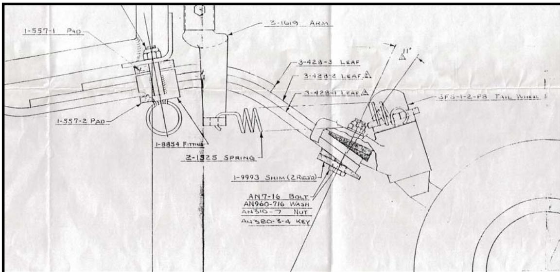
The next detail shows the details of the “Shim – Tailwheel – Maule” shown on n Champion Aircraft drawing 1-9993. The material of construction listed on the drawing was .38” X 1.50” X 1.50” 2024-T3, T4 Aluminum Sheet in accordance with specification QQ-A-362. The number required for assembly is 2 and the
