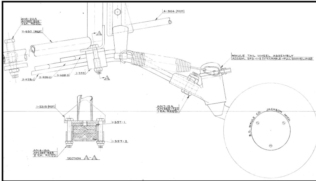
The photo shown below displays a portion of the installation shown on Champion Aircraft drawing 4-1423. for the Maule 3FS-1-2-8P pneumatic tired tailwheel.
